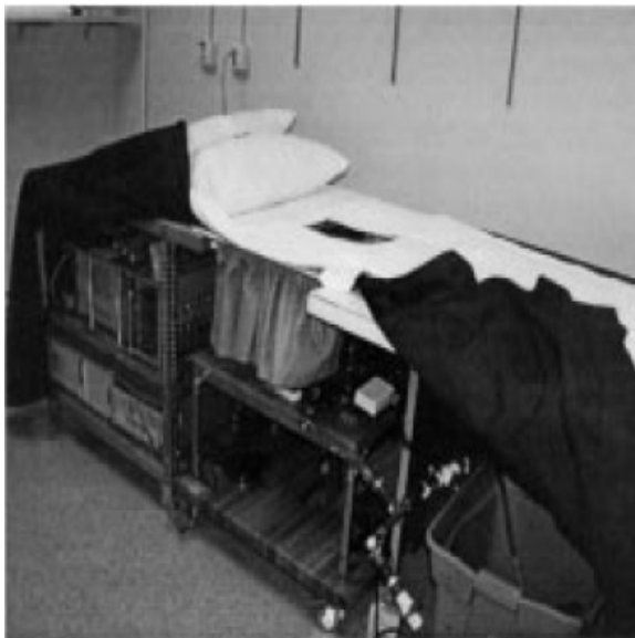
Figure 5: The clinical prototype for active microwave imaging of the breast in application of breast tumor detection, developed by Meaney et al. [25].
