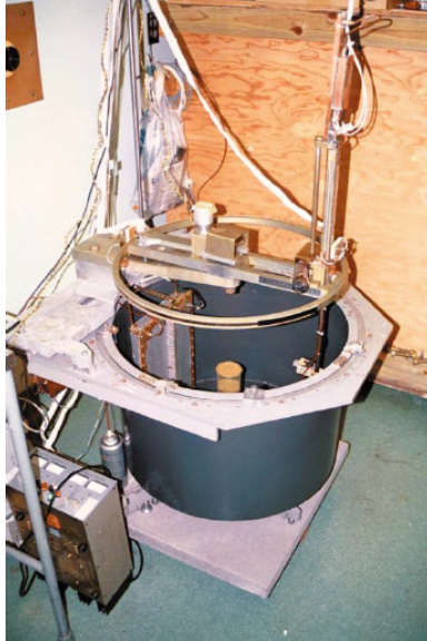
Figure 7: The first 3-D vectorial experimental setup developed by Semenov et al. [36], with a operating between 2.36 GHz.
