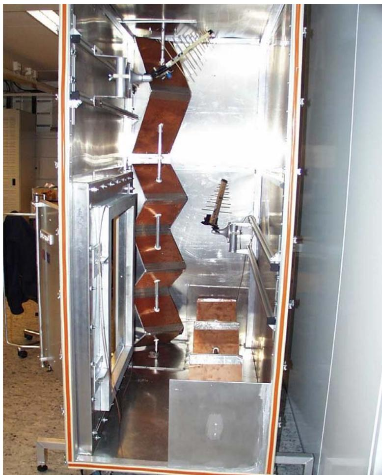
Figure 3. The interior of the RC at Flextronics, Linköping Sweden. The picture is taken from a side with a removable side wall and the dual stirrers made out of copper and the EMC-door (to the left).
