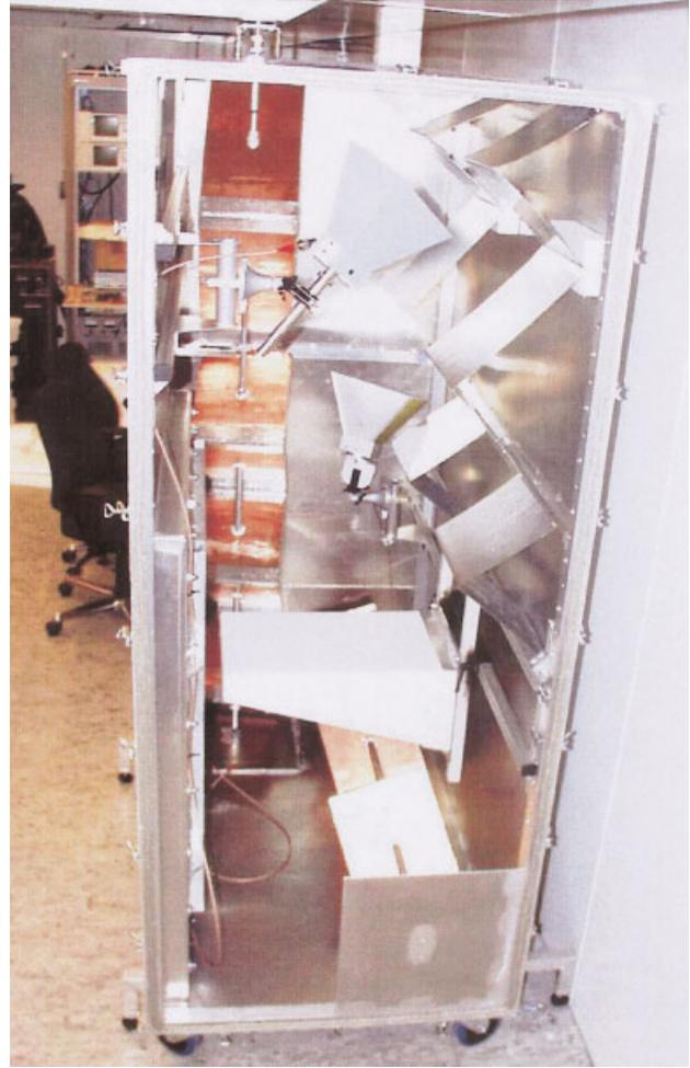
**Figure 1** Interior of the scattered field chamber (SFC). [Color figure can be viewed in the online issue, which is available at [www.interscience.wiley.com](http://www.interscience.wiley.com).]
