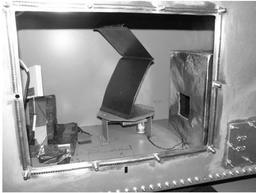
Figure 4. The interior of the small reverberation chamber used for the measurements. In this picture one can see the shielded anechoic box with apertures used to control the DOA of the plane waves [9] although it was not present in the chamber during the measurements presented here.
