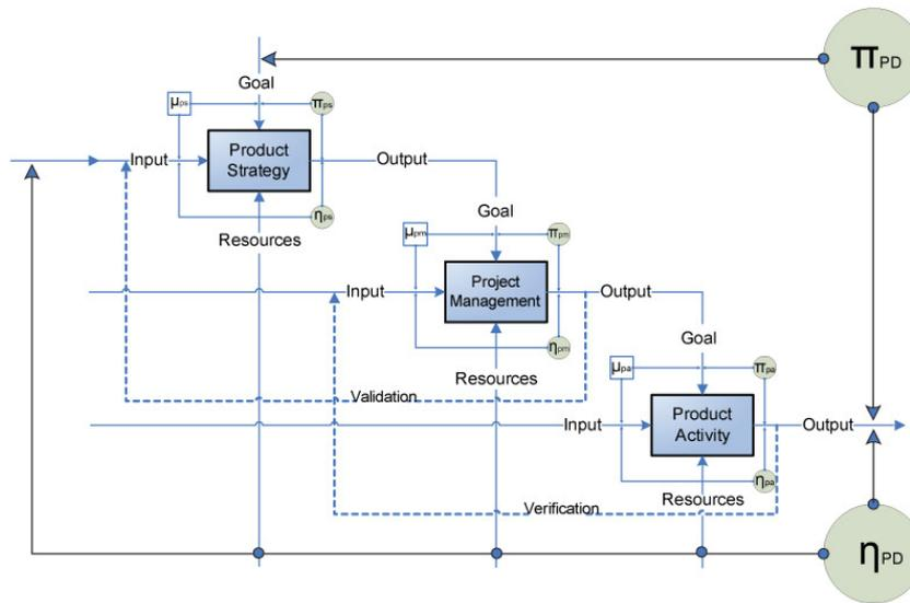
**Figure 2.** The proposed PDOPM model with the three generic levels of activities: product strategy, project management, and product activity. The relations of uncertainty ( $\mu$ ), effectiveness ( $\Pi$ ), and efficiency ( $\eta$ ) are also shown in the figure, both for each activity and for the complete PD process.
