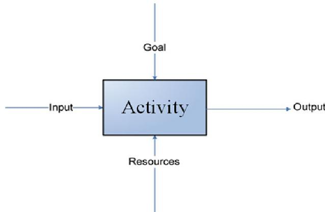
**Figure 3. An activity model based on the IDEF0 [43]**
