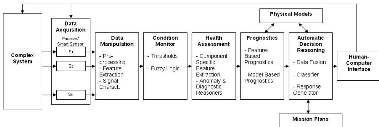
**Figure 4.** The seven modules in the OSA-CBM architecture standard proposal as presented in Lebold et.al (2003).
