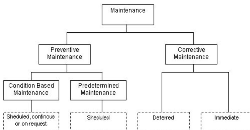
**Figure 1.** Overview of the different maintenance types (SS-EN 13306, 2001).
