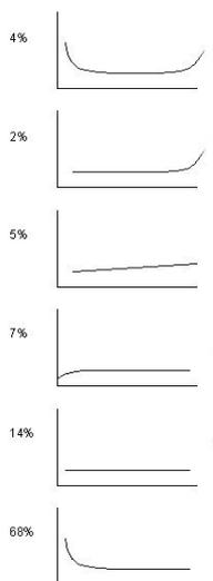
**Figure 3.** The six different conditional-probability curves generated by the United Airlines aircraft study.
