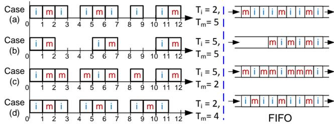
Fig. 6. Demonstration of maximum interference on  $m_m$  from the messages in the group  $M(m_m)$ .
