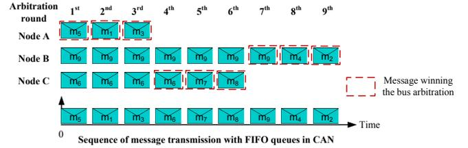
Fig. 5. CAN arbitration and FIFO-based queuing.
