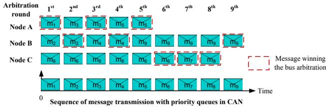
Fig. 4. Demonstration of CAN arbitration and priority-based queuing.
