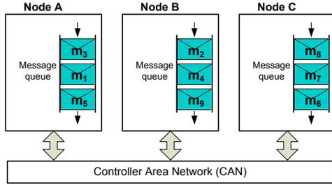
Fig. 3. Example to demonstrate the effect of queuing policy on message transmission.
