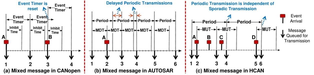
Fig. 2. Mixed transmission pattern in higher-level protocols for CAN.
