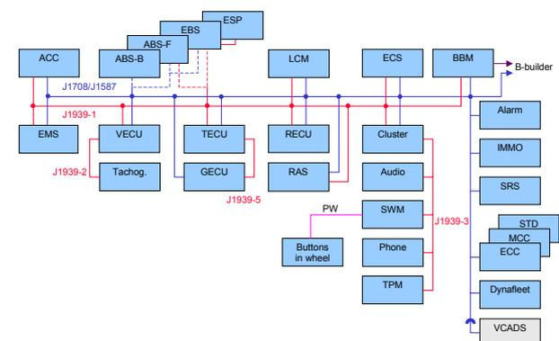
**Figure 2. Volvo FH electronic architecture.**
