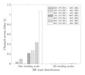
Fig. 3. Average channel access delay for MAC Protocol 1 for different loads and distributions of load.
