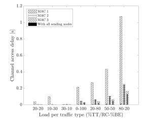
Fig. 8. Average channel access delay for the different MAC protocols under different loads and distributions of load. For MAC 2 and MAC 3, only the best configurations are shown (MAC 2B and MAC 3B). Thin black bars represent the case when traffic comes from all nodes.
