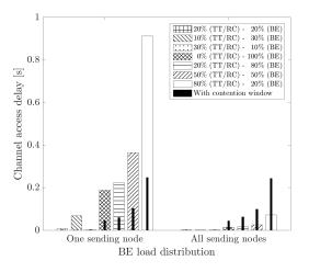
Fig. 4. Average channel access delay for MAC Protocol 2A for different loads and distributions of load. Thin black bars are for MAC 2B.
