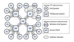
Fig. 1. Example of the proposed wired-wireless scenario, with switches (SW) and access points (AP) connecting the end-systems (ES, WES) forming recursive star topologies (snowflake topology). Note that every wired connection forms two collision domains, while the wireless systems constitute a single collision domain.
