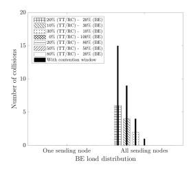
Fig. 5. Number of collisions for MAC Protocol 2A for different loads and distributions of load. Thin black bars are for MAC 2B.
