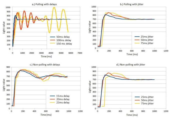
Fig. 6: System response under delay and jitter greater than sampling period, both polling (a and b) and non-polling (c and d) approaches.
