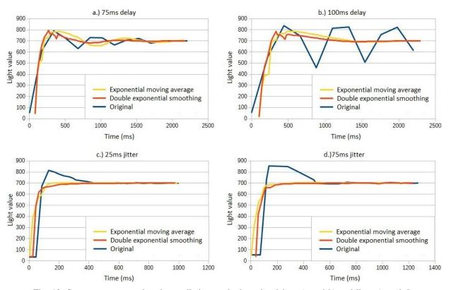
Fig. 12: System response using the prediction methods under delays (a and b) and jitter (c and d).
