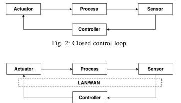
Fig. 3: Closed loop with networked controller.
