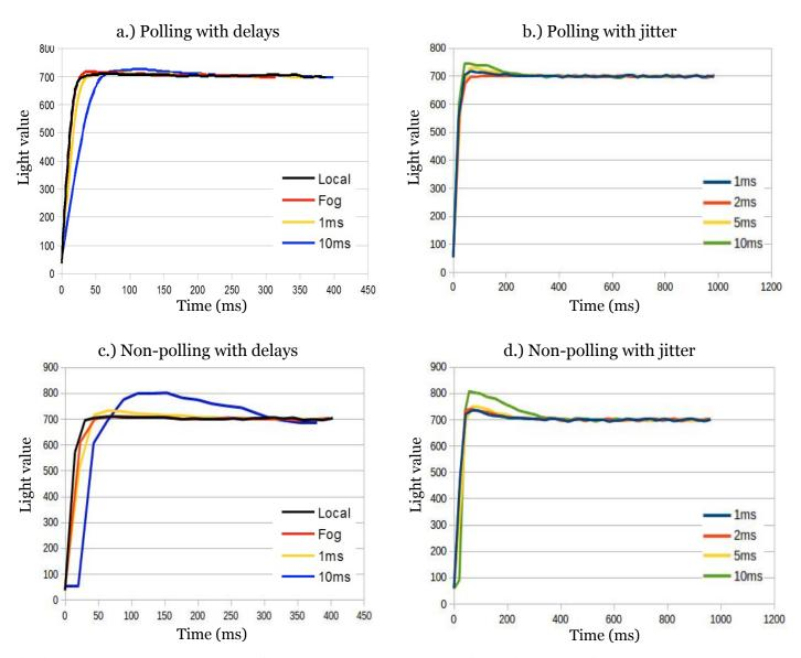
Fig. 5: System response under delay and jitter smaller than or equal to sampling period, both polling (a and b) and non-polling (c and d) approaches.
