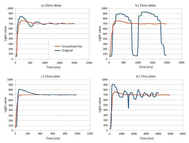
Fig. 11: System response using adaptive PI control under different delays (a and b) and jitter (c and d).
