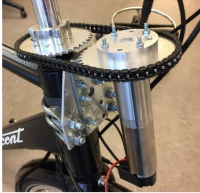
Figure 17: Image of the previous iterations motor mount with the plastic chain in place.
