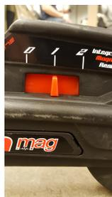
Figure 33: The analogue switch for the roller where the resistance can be changed during runtime.
