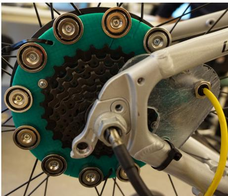
Figure 19: Twelve evenly distributed magnets used for speed measurement.
