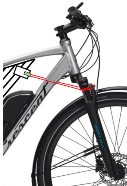
Figure 11: The soapbox string acting as a pulling force on the header, breaking the amplifier enable signal to the motor controller.
