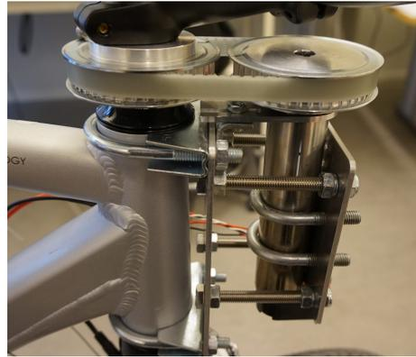
Figure 18: The steering motor mount with both cogwheels in place and the strap well tightened.
