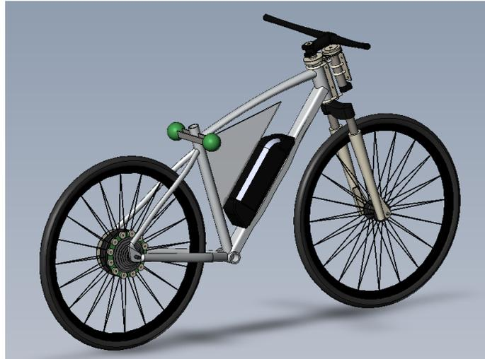
Figure 4: The SolidWorks CAD model of the bicycle used for extracting mass properties and running simulations.
