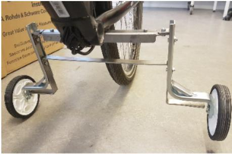
Figure 22: The final design of the support wheels built from the previous bicycle iteration.
