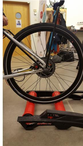
Figure 32: To further validate the speed controller, the back wheel was placed on a bicycle roller where the resistance of the roller can be changed during runtime.
