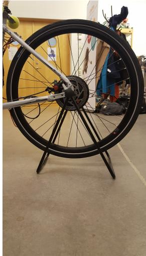
Figure 31: The first experimental setup to validate the speed control. In the first experiment the bicycle stands on a rack and the back wheel can revolve without friction.
