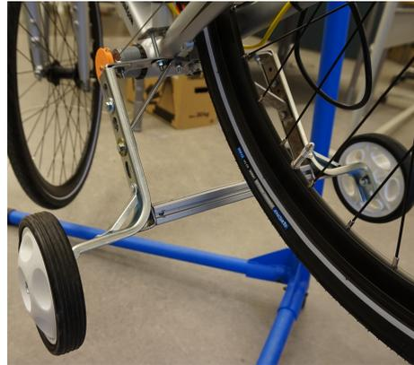
Figure 23: The new and improved version of the support wheels mounted on the bicycle.
