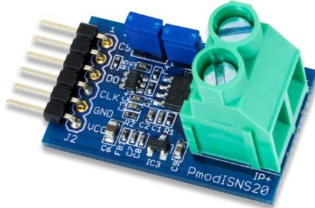
Figure 7: Picture of the current sensor PmodISNS20; this sensor is wired in series between the battery and the electrical system.
