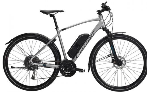
The Crescent ELis [41] has a rear-wheel drive electrical engine located in the rear wheel, a rechargeable 36V 11Ah battery located on the main frame, and a control panel on the front fork. The bicycle, which is a male model, comes in three sizes: 51, 55, and 59 cm. The downsides to the ELis model is that its adjustable handlebar is quite limited, and the Bafang motor controller has no official documentation.
