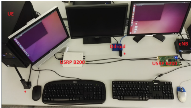
Fig. 4. Hardware setup of the LWA testbed implementation.
