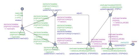
Fig. 13. The UTA template of dynamic obstacle initialization
