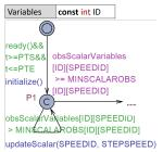
Fig. 9. A part of UTAI for initializing linear velocities of dynamic obstacles.
