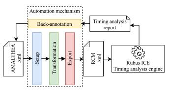
Figure 13: Overview of the automation mechanism and its phases.
