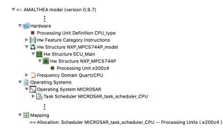
Figure 8: Extract of an AMALTHEA architecture depicting a ProcessingUnit element, a TaskScheduler element and the SchedulerAllocation element.
