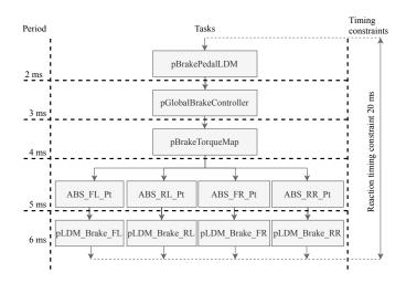
Figure 14: Block diagram of the BBW application. Different tasks and their communication pattern are shown. Task period and reaction time constraints are annotated.
