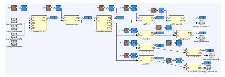
Figure 16: Excerpt of the RCM architecture of the BBW system realised within Rubus ICE.
