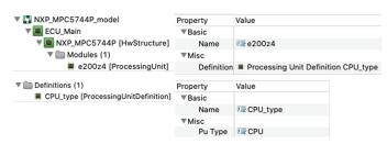
Figure 7: Extract of an AMALTHEA architecture depicting an Hw-Structure element, a ProcessingUnit element and their relationship.
