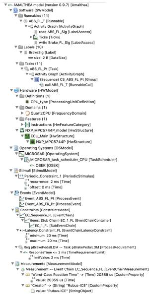
Figure 15: Excerpt of the AMALTHEA architecture of the BBW system realised within the Eclipse APP4MC platform.
