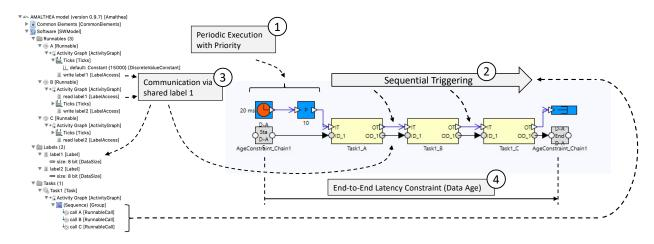
Figure 10: Extract of an AMALTHEA architecture and its RCM representation. Highlighted are the periodic execution with fixed priority (marking 1), mapping of runnable execution from AMALTHEA tasks to sequential execution in the RCM model (marking 2), communication via shared labels in the AMALTHEA model and mapping to communication via data channels in the RCM model (marking 3), and representation of end-to-end timing constraints in the RCM model (marking 4).
