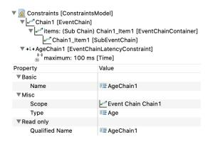
Figure 11: Extract of an AMALTHEA architecture depicting a latency data age constraint.
