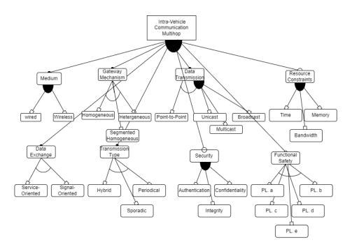
Fig. 9. Multi Hop Feature Diagram
