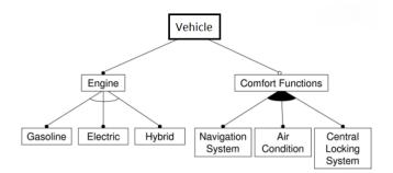
Fig. 6. An Example Feature Diagram
