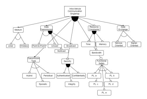
Fig. 8. Single Hop Feature Diagram
