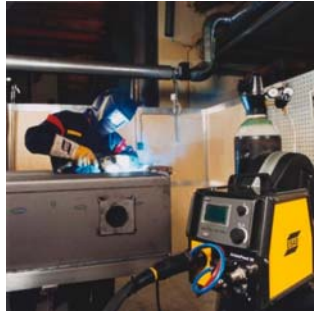
Fig. 1: Welding equipment with a CAN-based, distributed control-system
