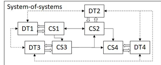
Fig. 3. A system-of-digital twins or distributed digital twins.
