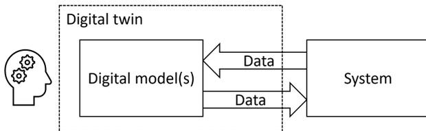
Fig. 1. A digital twin is the combination of data to and from the system, digital models of the relevant aspects, and the surrounding software needed for the operation.
