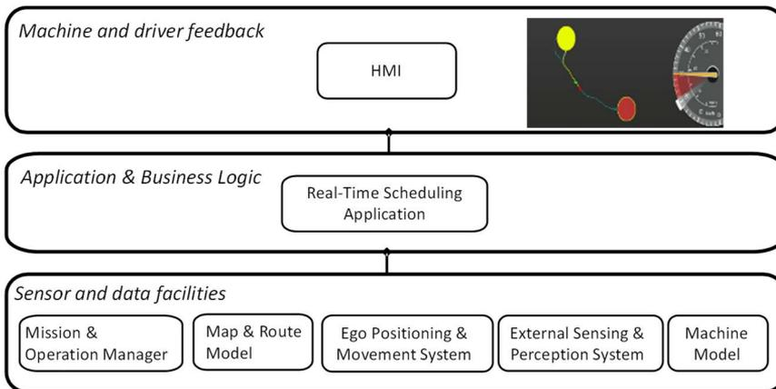
Figure 6. Machine internal SW component used in the study.
