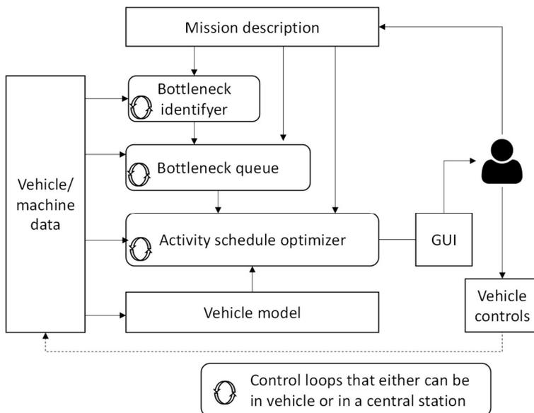
Figure 7: High level of logical components the control system presented.
