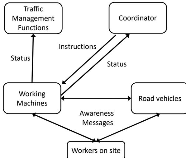
Figure 3. Road construction communication architecture.
