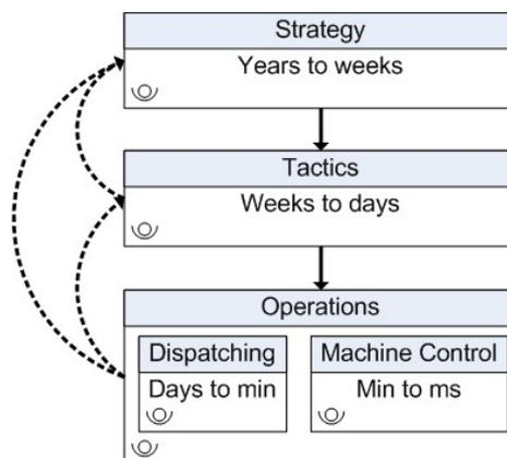
Figure 2. Levels and time horizon perspectives for site optimization and control with information feedback loops.
