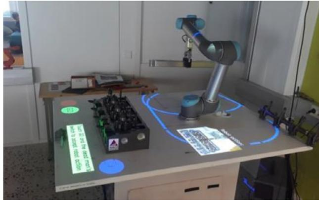
Fig. 8: Robot and AR-based UI using projector-mirror [36]
