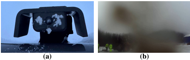
Fig. 2: Illustrative examples of (a) a dirty camera lens covered by e.g., snow, and (b) a recorded image with dirt-induced occlusion at a construction quarry.
