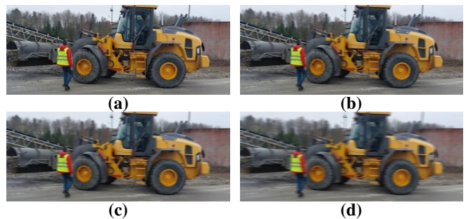
Fig. 1: Illustrative examples of linear motion blur with varying kernel sizes: (a) L = 3 , (b) L = 5 , (c) L = 7 , and (d) L = 11 .
