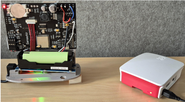
Fig. 1. Physical setup of the experimental system, showing the ESP32 microcontroller with an attached temperature sensor (positioned behind the board) and the Raspberry Pi configured as the edge/fog node.
