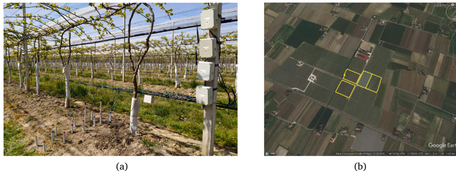
Fig. 3. A sensor grid (left) monitoring soil moisture close to a kiwi tree in a commercial orchard located in Faenza, Italy (right). The watering system is composed of single-pipeline drippers.
