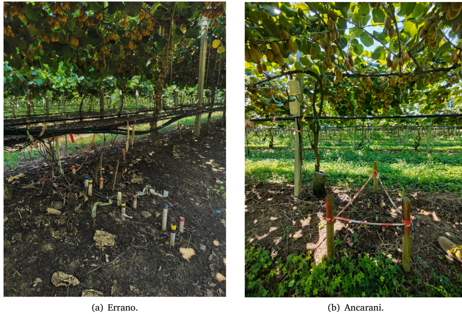
Fig. 13. Settings of the field experiments in two commercial orchards. Two-dimensional grids of gypsum block sensors are deployed to measure soil moisture, and drippers are automatically controlled by SMARTER: (a) a grid of 4 columns of 3 sensors has been installed, and (b) a grid of 3 columns of 3 sensors has been installed.
