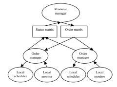
Figure 2: Information flow between Matrix's components
