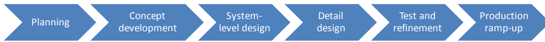
Fig. 1. The generic phases in the PD process involve planning, concept development, system-level design, detail design, test and refinement, and production ramp-up [10].
