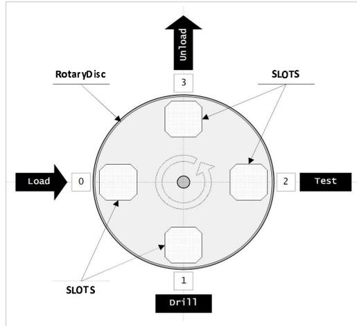
Figure 8. Schematic diagram of a Turntable system
