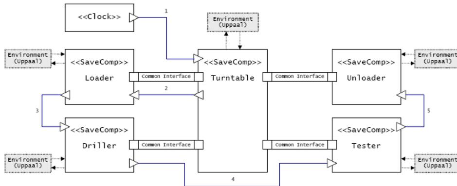
Figure 9. Software architecture design layout of Turntable system
