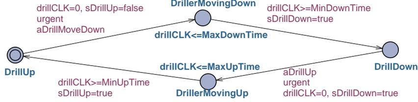
Figure 18. Behavior of Drill of the environment model.
