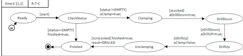
Figure 13. State machine model of the Driller component.
