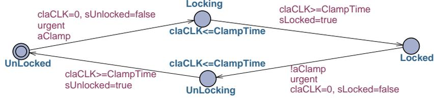
Figure 17. Behavior of the Clamp environment model.
