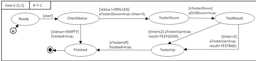
Figure 14. State machine model of the Tester component.
