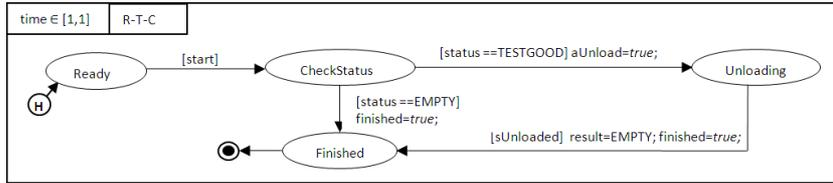
Figure 15. State machine model of the Unloader component.
