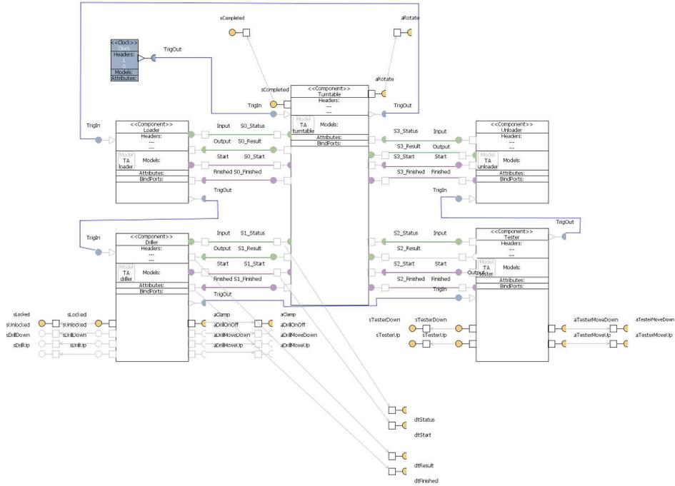
Figure 16. Control structure and system architecture of the turntable system as modeled in Save-IDE.
