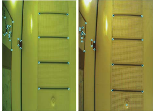
Figure 2. A photo of the ceiling and corner features extracted using Harris and Stephens combined corner and edge detector, the corners are clustered with a 10 pixel radius.
