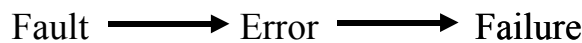
Figure 2-1. Cause-consequence diagram of fault, error and failure. Where the failure signifies a behavior non-compliant with the specification. Where an error signifies a state that can lead to a failure, and where the fault is the hypothesized cause for the error.
