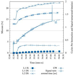
Figure 2: Cache misses and CPI when running a simple signalling application bouncing signals between two processes located on the same core. The load regulation application strives to have a system miss rate of 0.74% L1 I-cache, 3.3% L1 D-cache and 22% L2 D-cache which is similar to a production system. The regulation scenario described in this figure was started after the system was completely stable, in our case after about 52:00 minutes
