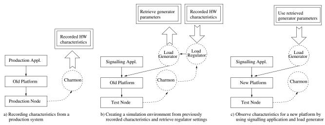
Figure 1: Our procedure in three steps to measure characteristics for a new software release by modelling a production system.
