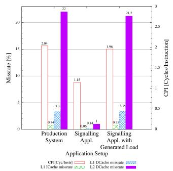
Figure 3: Measured cache usage and CPI for the reference system, test application and a recreated execution environment with the test application. Characteristics for the reference system is similar to the mimicked scenario.
