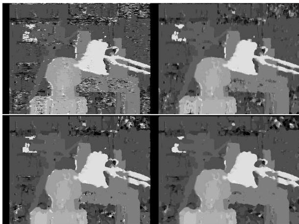
Figure 4: The median filter (right column) significantly reduces the noise for the 1D (top) but not the 2D (bottom) approach.
