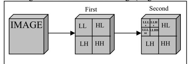
Fig. 1: Two-dimensional wavelet transform for an image
