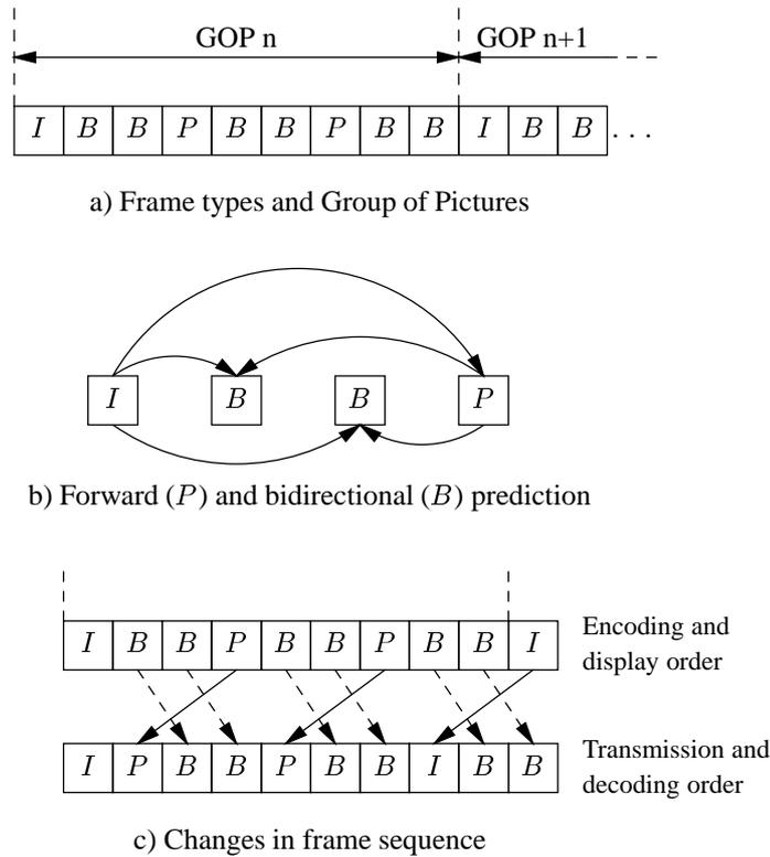
Figure 1: MPEG-2 video stream characteristics
