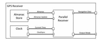
Fig. 2. A simple GPS receiver component.
