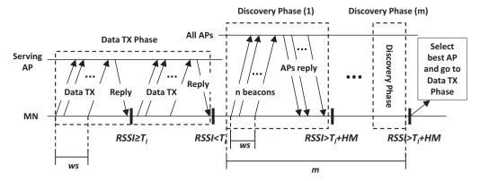
Fig. 2. Timing diagram of the smart-HOP mechanism.
