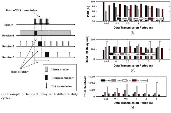
**Fig. 10.** Impact of network duty cycling on mRPL performance with different network traffics: (a) an example of hand-off delay with different duty cycles, and performance in terms of (b) packet delivery ratio, (c) average hand-off delay, and (d) total packet overhead.
