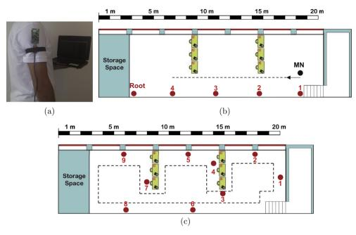
Fig. 12. Experimental evaluation, (a) the MN attached to the shoulder, (b) Experimental Setup 1 with 4 APs and a MN deployed in a row, and (c) Experimental Setup 2 with 9 APs distributed across the lab.
