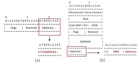
**Fig. 4.** (a) The modified DIS packet format. Two fields of *F-DIS* and *C* are added to the RPL DIS packet, and (b) the modified DIO packet format. Two fields of *F-DIO* and ARSSI are added to the RPL DIO packet. Additional bits are applied to the "Option(s)" part of the packet.
