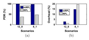
Fig. 14. Compare RPL and mRPL in terms of (a) PDR and (b) overhead in Experimental Setup 1.
