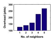
Fig. 11. Impact of network density on total overhead.
