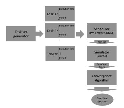
Fig. 1: Overall scheme of task set simulator
