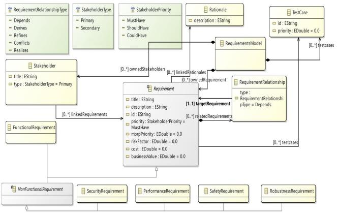
Fig. 1 Meta-model for requirements and test case prioritization
