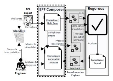
Figure 7.1: Automated Compliance Checking Vision.
