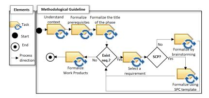
Figure 10.2: Methodological Guidelines to formalize ISO 26262 into FCL.
