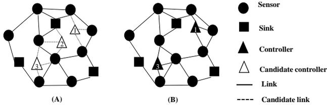
**Figure 2.** An illustrating example for the controller selection [4].
