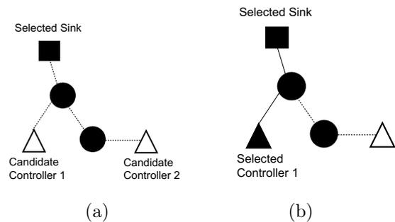
**Figure 3.** An example of controller selection with respect to a selected sink; (a) a scenario with two candidate controllers, and (b) the selected controller with respect to the  $l'_{max} \leq 2$  constraint [4].
