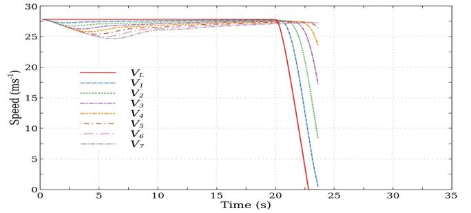
(a) ACC with normal braking ( $-12ms^{-2}$ )
