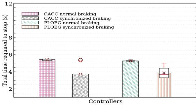
Fig. 7. Total time required for the platoon to come into complete standstill for different controllers.
