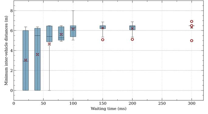
Fig. 3. Minimum inter-vehicle distances for different waiting times for a platoon of length 8 cruising at a speed of 100 kmh<sup>-1</sup> with an initial inter-vehicle distance of 8 meters.
