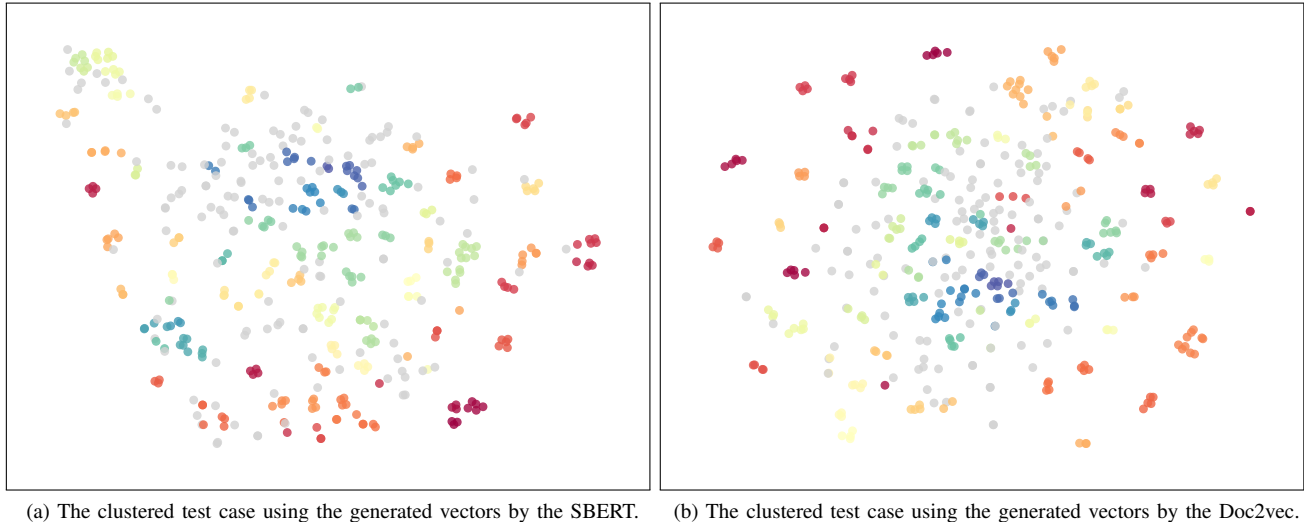
Figure 5. The clustered test cases using HDBSCAN algorithm on the generated vectors by two deep learning algorithms. There are 75 and 76 clusters plotted in different colors for SBERT and Doc2vec respectively. The outliers are shown in gray.
