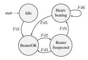
Fig. 1. Failure detection state machine.
