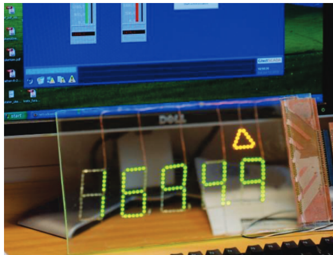
Figure 3. The image shows the transparent display prototype that was developed by Kvalberg [19]. The number indicates the current load that is lifted by an off-shore crane, while the yellow triangle indicates that the lifting load exceeds the permissible limit.
