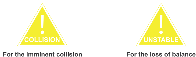
Figure 18. Two kinds of the warning sign. The left one is for when a collision is imminent to occur and the right one is for when the machine is about to tip over.
