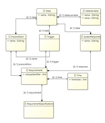
Figure 2: Meta-model for Gherkin-like DSL
