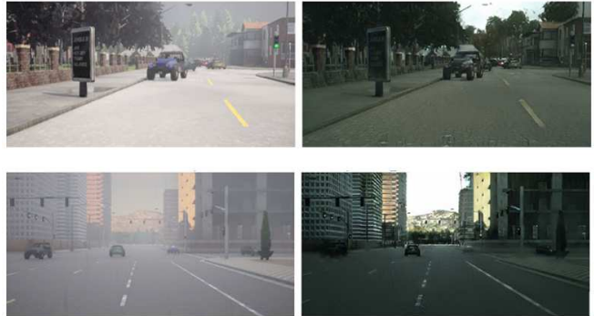
Fig. 16 Domain adaptation transformation from simulated environment with the CARLA simulator (left) to the real-world captured Cityscapes domain (German cities).
