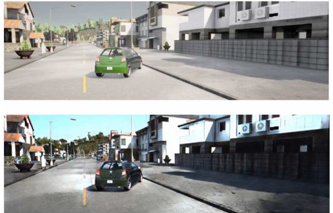
Fig. 15 Domain adaptation transformation from simulated environment with the CARLA simulator (top) to the real-world captured KITTI domain. Presumably, black cars are more common in real-world German cities than in our simulations where vehicle color was uniformly randomized.
