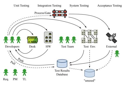
**Figure 1:** Automated system-level software testing of industrial networked embedded systems.
