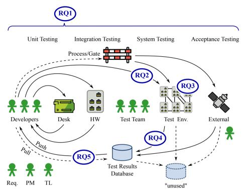
**Figure 2.1:** Automated System-Level Software Testing of Industrial Networked Embedded Systems with highlighted research questions (compare Figure 1).
