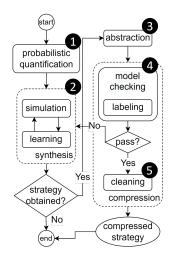
The workflow of MoCReL is shown in Fig. 4. Step 1: A probabilistic quantification is conducted on the TG to facilitate sampling over the system, effectively turning the TG into an STG (Stochastic Timed Game).
