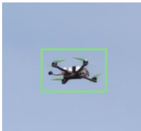
Figure 12 – The MobileNet V2 network identifies a drone in the zoomed in area ( AoU plus additional pixels). It identifies the drone with a confidence of 0.942.
