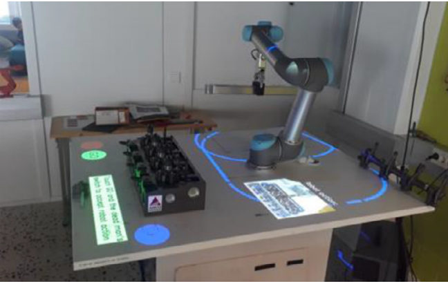
Fig. 7. Robot and AR-based UI using projector-mirror [35].
