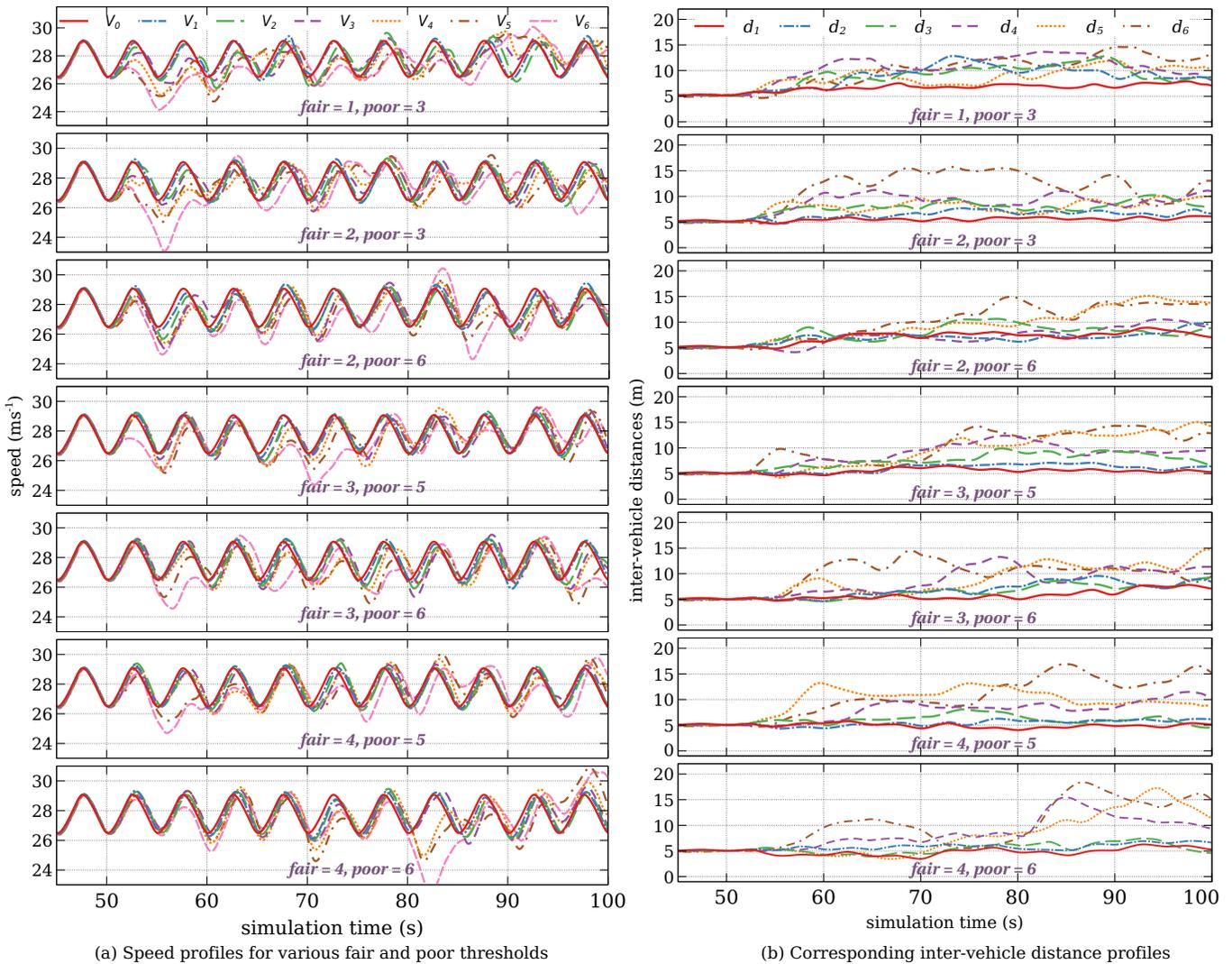
Fig. 7: Speed ( $\text{ms}^{-1}$ ) and inter-vehicle distance (m) profiles during cruising in a *sinusoidal scenario* for various *fair*, *poor* thresholds using the GDU method; oscillation frequency = 0.2 Hz, oscillation amplitude =  $10 \text{ km}^{-1}$ , ACC CTG = 1.2 s, CACC CTG = 0.5 s, PLATOON CDG = 5 m, speed =  $100 \text{ kmh}^{-1}$ .
