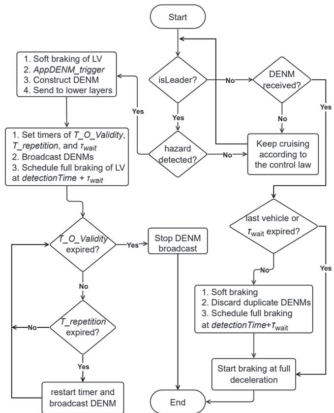
Fig. 4: Enhanced Synchronized Braking strategy.
