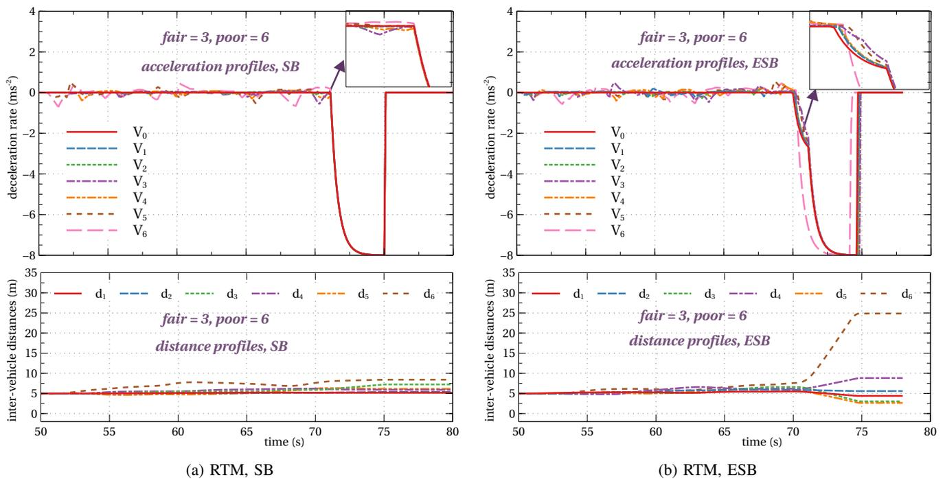
Fig. 9: Acceleration ( $\text{ms}^{-2}$ ) and distance (m) profiles using the RTM module with the SB and ESB strategies for the same configurations as in Table VII; the results of one simulation run ( $\text{fair} = 3$ ,  $\text{poor} = 6$ ) are presented.
