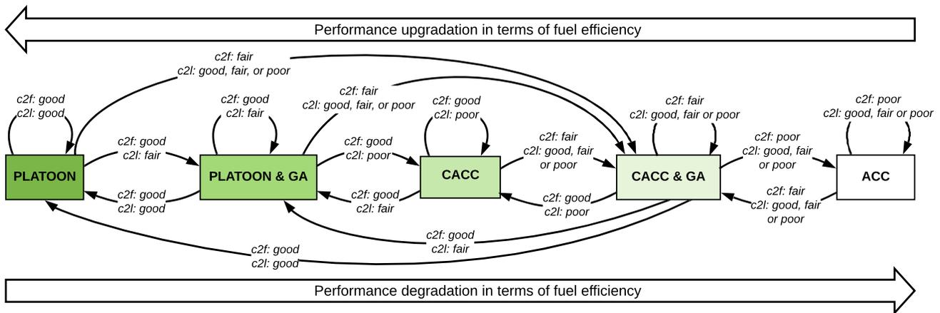
Fig. 2: Elaboration of the *Cruising States* representing the graceful degradation and upgradation method.
