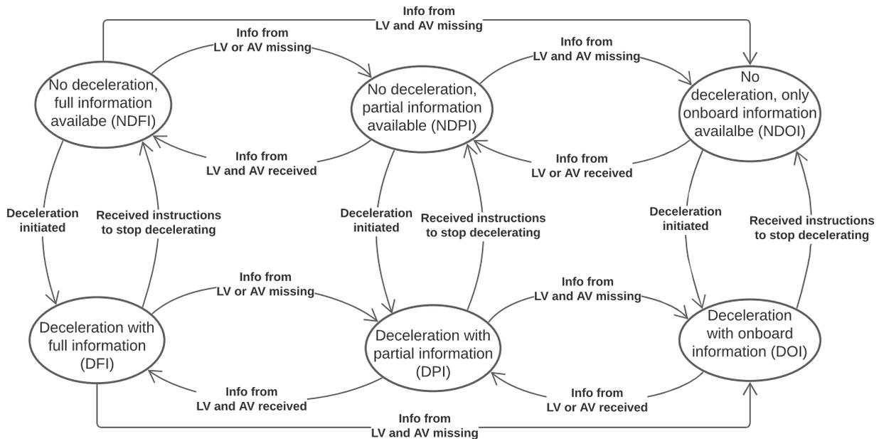
Fig. 3: Elaboration of the *Emergency Braking* states representing a general framework for different types of braking strategies.
