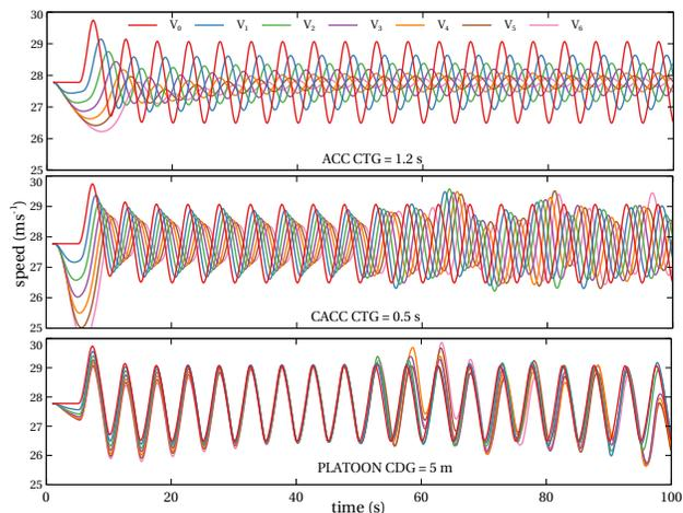
Fig. 5: The speed profiles of the vehicles in a sinusoidal scenario with ACC, CACC, and PLATOON controllers and no RTM; oscillation frequency = 0.2 Hz, oscillation amplitude = 10 km<sup>-1</sup>, ACC CTG = 1.2 s (35.35 m at 100 kmh<sup>-1</sup>), CACC CTG = 0.5 s (15.89 m at 100 kmh<sup>-1</sup>), PLATOON CDG = 5 m, speed = 100 kmh<sup>-1</sup>.
