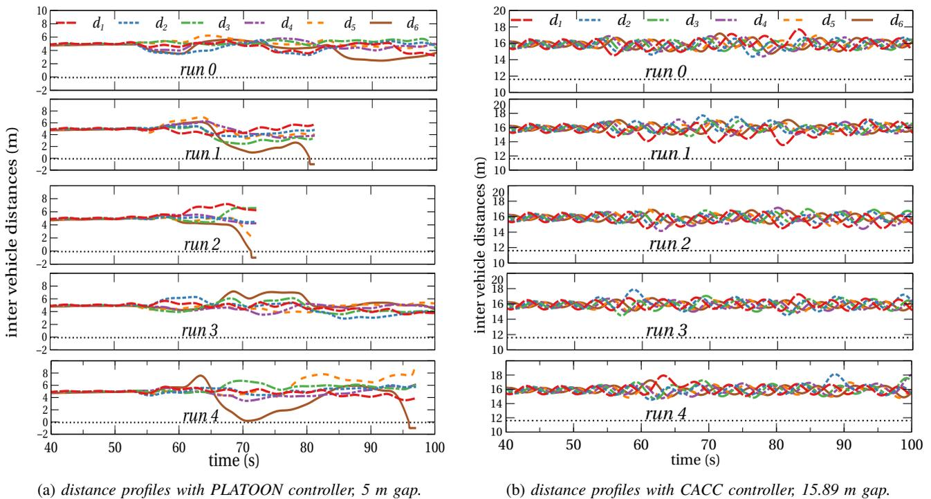
Fig. 6: Inter-vehicle distances in meters during cruising in a sinusoidal scenario with PLATOON and CACC controllers and no RTM in play; oscillation frequency = 0.2 Hz, oscillation amplitude = 10 kmh<sup>-1</sup>, (a) PLATOON CDG = 5 m, (b) CACC CTG = 0.5 s, i.e., 15.89 m at 100 kmh<sup>-1</sup>, speed = 100 kmh<sup>-1</sup>.
