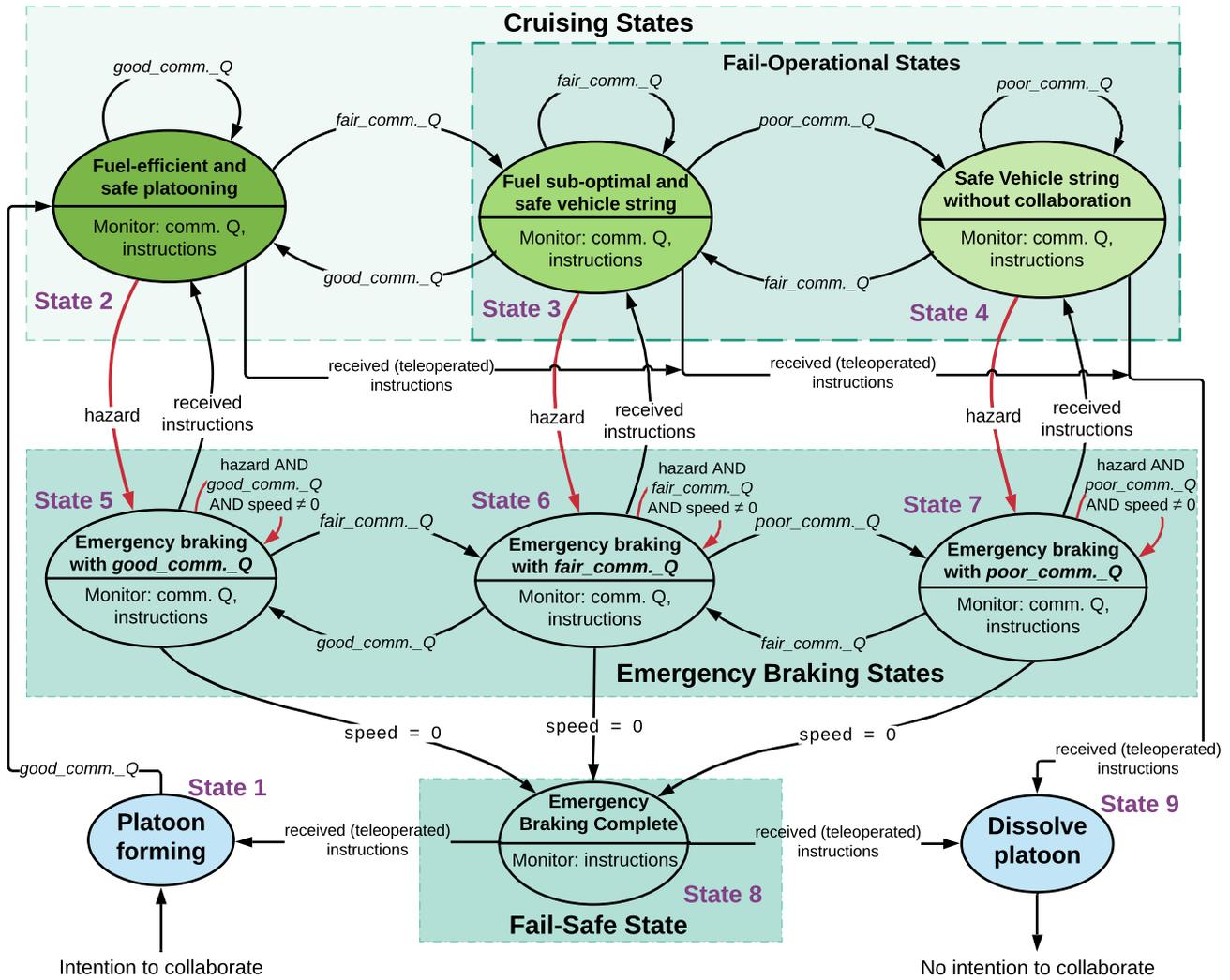
Fig. 1: State machine representing different states during platooning operation and the transitions between the states due to transient communication errors or road hazards.
