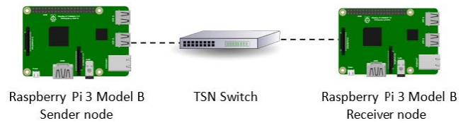
FIGURE 6. Heterogeneous TSN network with legacy end-stations topology.
