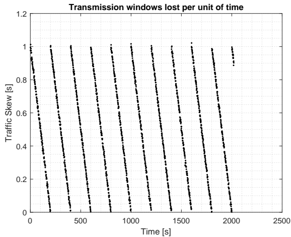
FIGURE 9. Traffic skew due to negative clock drift.
