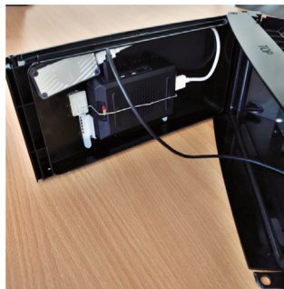
Fig. 7. Chamber of the smart traffic light with a Raspberry Pi [160].
