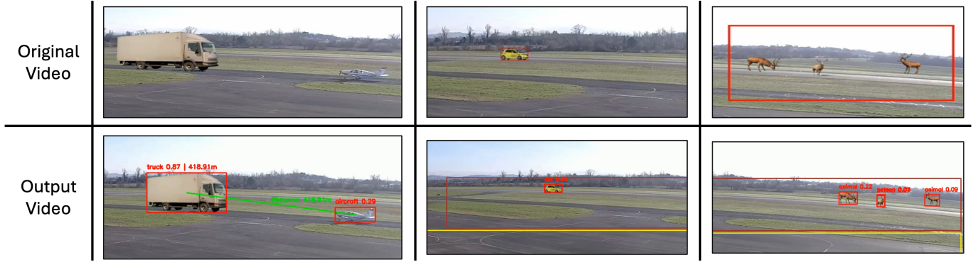
Fig. 4. Result of object detection within the region of interests.
