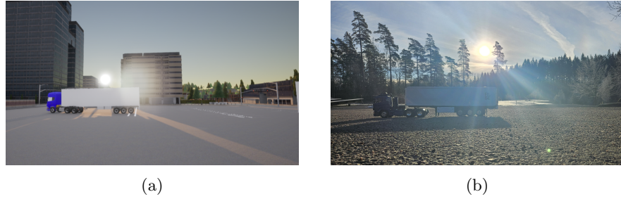
Fig. 4: Illustration of low sun glare test scenarios: the simulation environment shown in (a) uses CARLA with a sun elevation of 6^\circ , while the hardware-in-the-loop scale truck setup in (b) has a sun elevation of 9^\circ .
